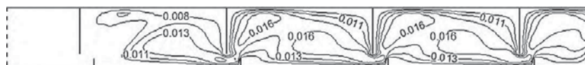
Fig. 6. Eddy viscosity (m 2 /s) computed by the numerical model in the design D4.10 with S = 5\% .
