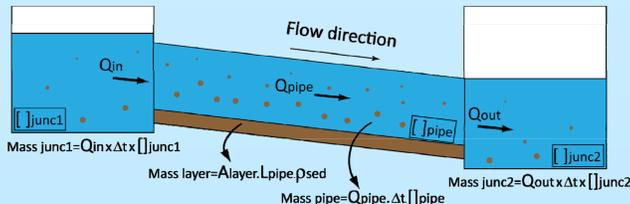
Figure 3. Mass availability in the different elements of the sewer network
