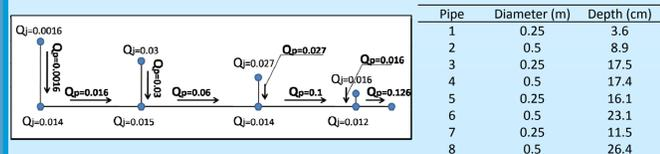
Figure 6. Sewer network water discharges (m3/s) Table 1. Pipe diameters and water depths
