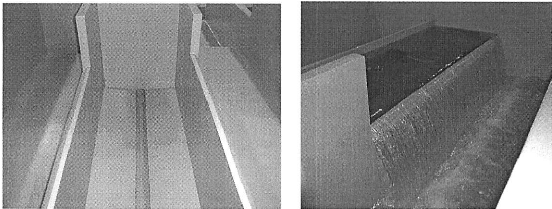
Fig 1.- Scale model of the first flush tank
