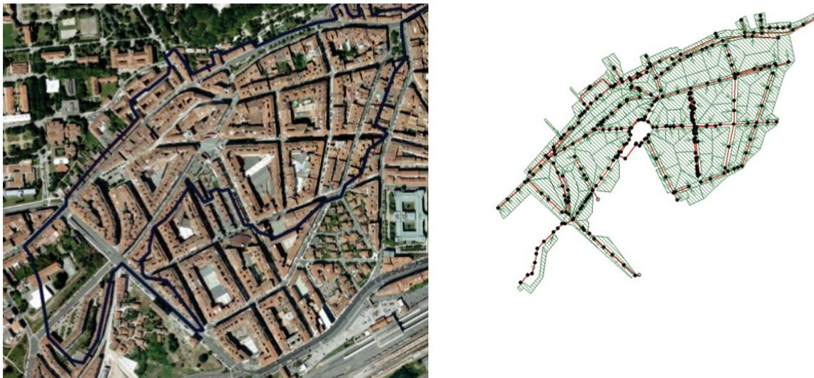
**Figure 1.** Layout of the El Ensanche catchment and the Infoworks CS distributed model.
