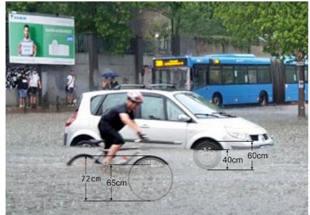
Fig. 4. Estimation of water depth using reference objects with an example of the challenge of local topographic heterogeneity. Estimating the water depth at the bike wheel in the foreground results in approx. 25 cm difference in water depth when compared to an estimation at the car wheel. Perhaps the biker is in a lower part of the road?
